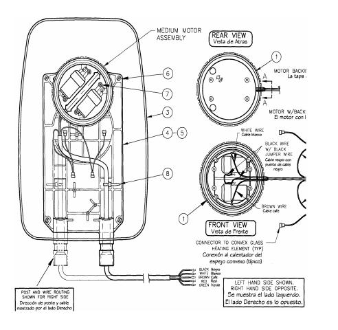
The drawing on the left is a cutaway view of a common Velvac mirror head. Inside the medium motor assembly are the cylindrical motors. To the right of the head is a rear and front view of the medium motor assembly.
