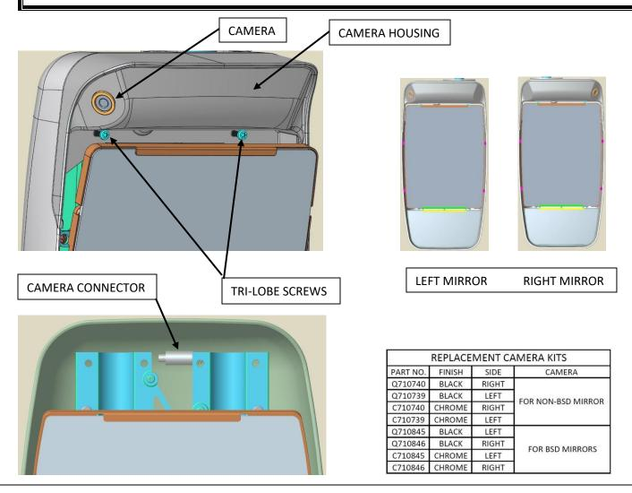
TOOLS REQUIRED: T20 TORQUE BIT WITH MAGNETIC DRIVER
